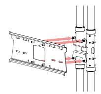
Push the column assembly into the top sockets, then over bottom bushes. Ensure the fixing holes align and using the through bolts, secure the columns into place. Tighten any grub screws at the rear.
