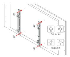
Utilising the grip locks (top), tag locks (bottom) and fixing pack provided with your mount, attach the arms to the back of your screen.
