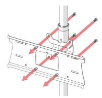
Push the column assembly into the top socket, then over bottom bush. Ensure the fixing holes align and using the through bolt, secure the column into place. Tighten any grub screws at the rear.
