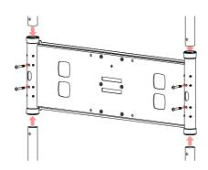
Cut columns to desired length so span-bar is at the correct height for the screen. Fit columns into sockets, top and bottom, either end of the spanbar. Feed cables through columns and out through aperture in socket. Secure with the through bolts provided and tighten grub screws.
