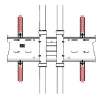
Once centred, ensure the bottom screws are not screwed tight and screw down the top screws to level the screen. Once level tighten bottom screws to secure the mount. ALT: If using tilting arms, this is when you can adjust them to suit.
