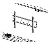
Screen mount incorporated into the housing backplate.
